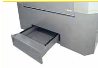
Collecting box for parts removable and transportable
