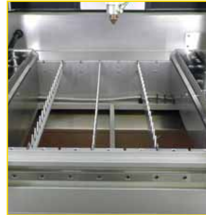
Front loading cutting box with plate tensioning and locking, pneumatic and manual clamps on fakir bed
