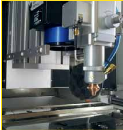
Combined application with integrated laser cutting and marker
