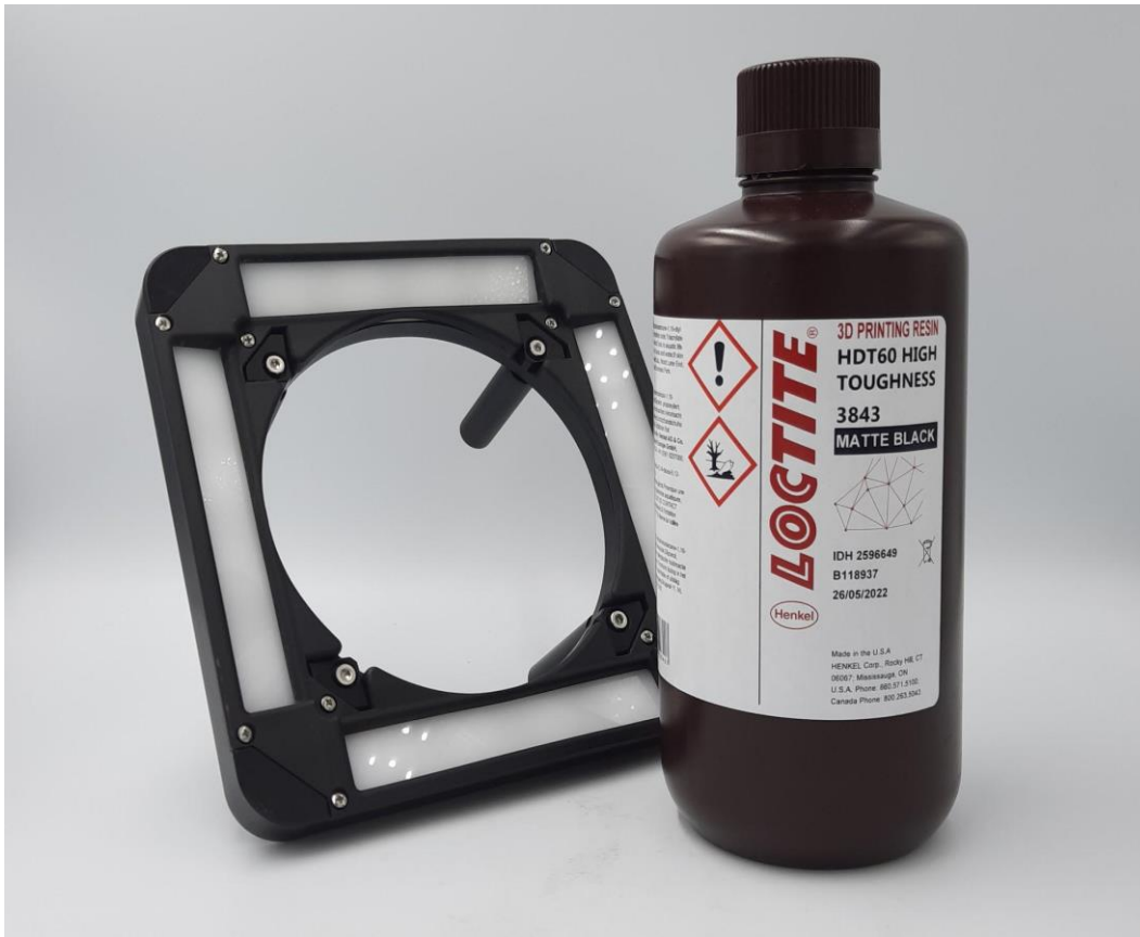
Sisma Spa laser marking machine part manufactured with Loctite 3D 3843 HT60 High Toughness resin on Everes DLP printer
