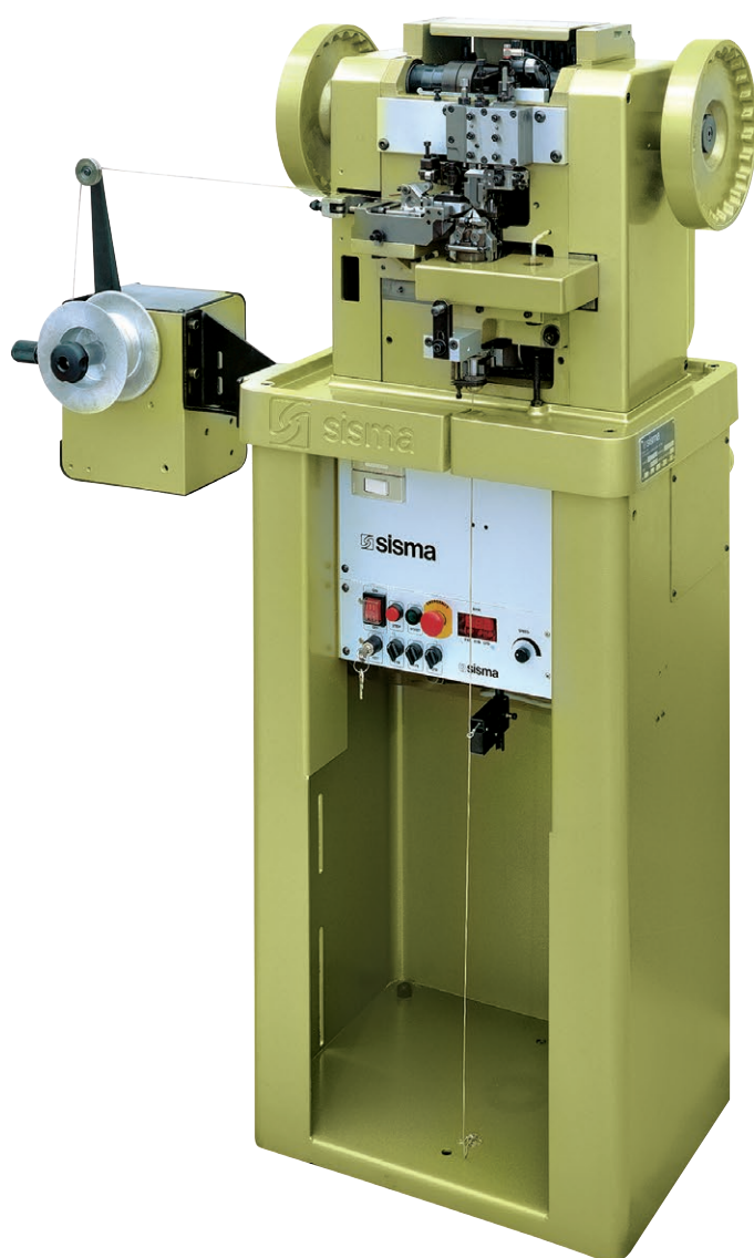
Automatic chain making machine for small venetian chains production
